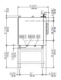
Cold Water inlet 1 (cleaning) CWII EI = Electrical inlet (power) = Cold Water Inlet 2 (steam generator)
